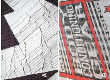
A.) Shatter Base is a new plastisol that was developed to easily crack apart. In this print, white ink made with Shatter Base was printed through an 86-thread/in. mesh, flashed, and printed a second time through a 110-thread/in. mesh to build up the proper amount of ink and produce a smooth surface. The print was cured with a moderate amount of extra heat. The combination of proper ink deposit and sufficient heat produce a graphic that feels brittle and cracks apart fairly easily.
