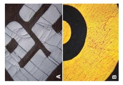
A.) A gray water-based ink formulated for cracking was printed through a screen with a low mesh count, flashed, and then overprinted again to build a sufficient ink-film thickness. The cured print cracks apart easily when it's bent or lightly stretched.
